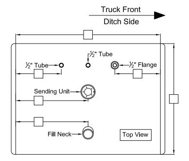
Please note: All sizes are NPTF unless otherwise noted and reference all measurements from the lateral weld seam and the end cap weld seam to the center of the fittings.
